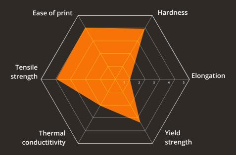
Martensitic stainless steel type 17-4 PH is hardenable by precipitation and show excellent mechanical properties. Gaz atomised starting powder maximal granulometry is 22 um. 17-4 PH is the preferred choice for severe applications where resistance to corrosion and high mechanical properties are required.
