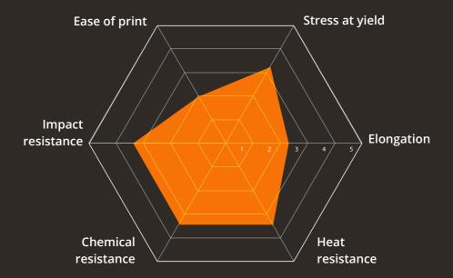
Polyamide 6-6 is a semi-crystalline thermoplastic and is the strongest unreinforced aliphatic nylon and the most resistant to abrasion and low temperatures. It has good resistance to friction and impact. PA6-6 can be alloyed with fiberglass or carbon and used as reinforcement materials.
