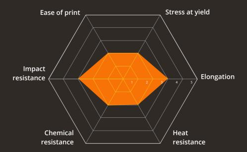
PBT belongs to the family of polyesters. This semi-crystalline polymer has good electrical insulating properties, excellent heat resistance, good resistance to chemical agents. It is imperative to dry the material properly before processing. Compared to PET, PBT has slightly lower strength and rigidity, slightly better impact resistance, and a slightly lower glass transition temperature.
