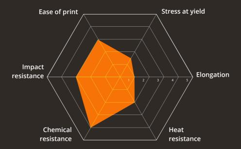
PE is a semi-cristalline polyolefin. Classified by its density and branching, PE properties depend of their molecular weight and structure (cristalline).
