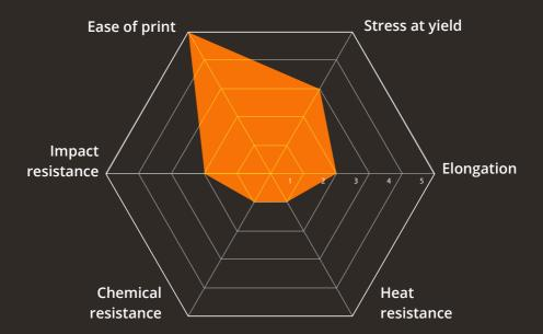
PLA is a semi-cristalline bio-based polymer obtained from renewable ressources. It is a copolyester massively used in 3D printing for prototypes fabrication.
