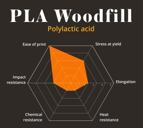
PLA is a semi-cristalline bio-based polymer obtained from renewable ressources. It is a copolyester massively used in 3D printing for prototypes fabrication. Wood fiber filled PLA presents a nice woody aspect. Many other types of filling exist.
