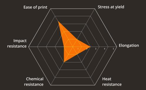
PVOH is a water soluble thermoplastic mostly used for its film forming, adhesive and emulsifying properties. It presents good mechanical properties and resistance to oil and grease but loose its performances in contact with humidity or water acting as a plasticiser. Mainly used as sacrificial material for support structures in 3D printing process, it is compatible with PLA and any other polar polymers in general.
