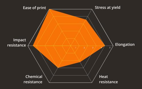
TPE Ultra Flex is a translucent, super-soft grade present. It is easy processing, dry surface, excellent mechanical properties at low hardness and pleasant surface feel (soft touch) and is Suitable for food contact applications. This TPE High Flexibility has a good adhesion with PP.
