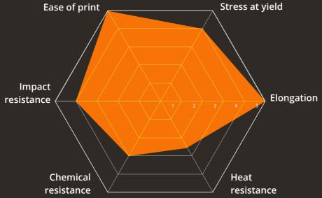
TPE High Flexibility is a translucent colored grade. It exhibits excellent compression set, excellent mechanical properties, high elasticity and perfect surface finish and is suitable for food contact applications. This TPE High Flexibility has a good adhesion with PP.
