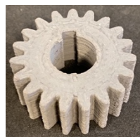
Figure 11 - Gear 3D printed in Low alloy steel - 8620
