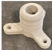
Figure 10 - Tripod 3D printed in Titanium - Ti6Al4V
