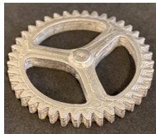
Figure 9 - Gear 3D printed in Stainless Steel - 17-4 PH
