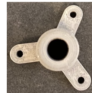
Figure 10 - Tripod 3D printed in Titanium - Ti6Al4V
