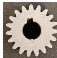
Figure 11 - Gear 3D printed in Low alloy steel - 8620
