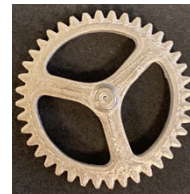
Figure 9 - Gear 3D printed in Stainless Steel - 17-4 PH
